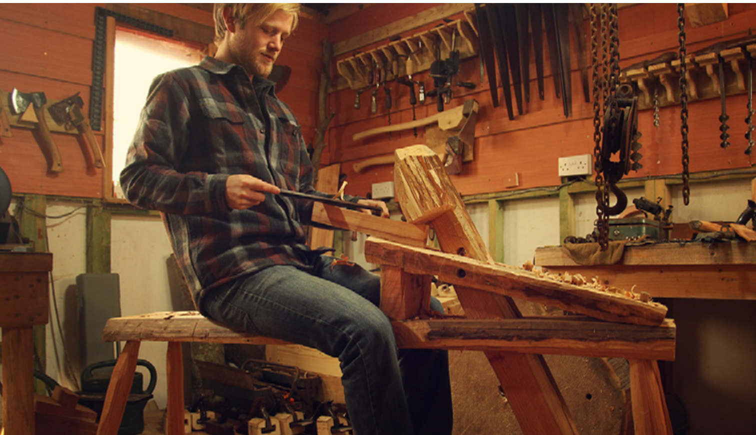
Above: Eamonn O'Sullivan. Shaving with a drawknife and a shaving horse (or coopers mare). November 2014. Hewn.ie. https://www.hewn.ie/blog-content/2014/10/29/what-is-green-woodworking/
